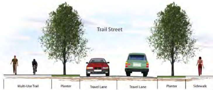
Figure 6.21 Possible trail street section
