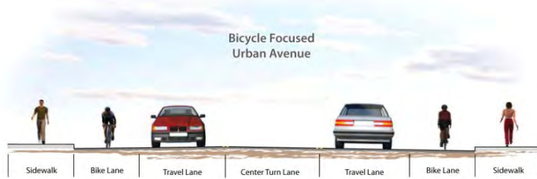
Figure 6.16 Possible Bicycle Focused Urban Avenue section
