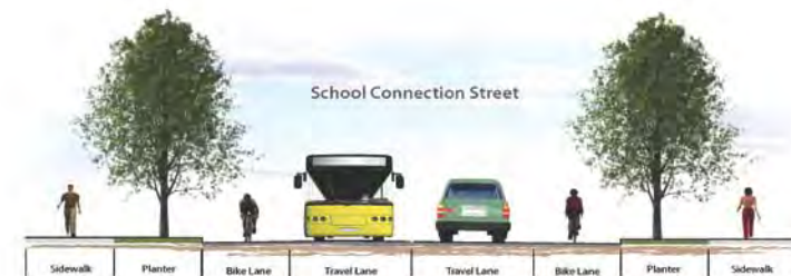
Figure 6.19 Possible school connection street section
